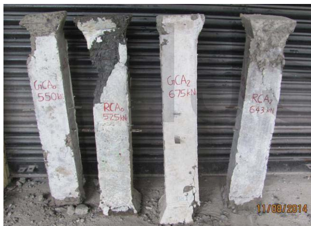
Fig. 3. Tested column specimens
